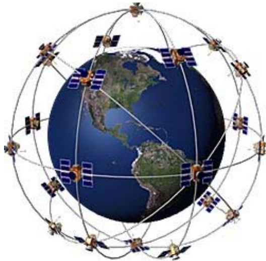
Figure 1: GPS Satellite Constellation, [GARM05] © Garmin Corp. 2005.
